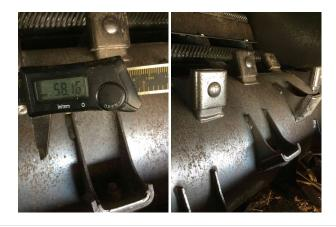
• 5.19 Inspect threshing cylinder (Inc. rasp bars and filler plates (option)
