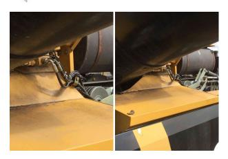
9.21 Inspect grain tank fill auger and the cross augers/covers in the grain tank for excessive wear of damaged flighting
