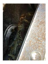
9.32 Inspect impeller drum and wear plates (option) for excessive wear or damage. measure and record height of impeller paddles on the outside and inside areas.
