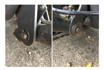
5.37 Inspect feederhouse dampening springs or accumulators/valve. Machines equipped with accumulators, Check accumulator pressures with feederhouse resting on locks.
