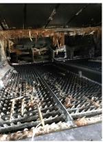
7.6 Inspect sieve linear adjustment motors, linkage, connectors and wiring
