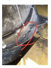
6.38 Inspect the elbow of the unloading auger for cracks or broken hardware
