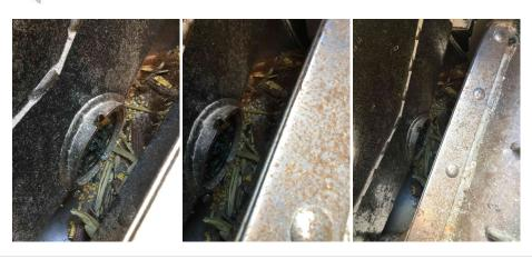
9.31 Check rotor bearings to make sure they are full of good grease and free of dirt/chaff build up
